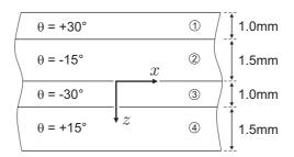
**4.** For each of the laminates below, describe the deformation under a unidirectional traction  $N_x$  and under a bending moment  $M_x$ .
