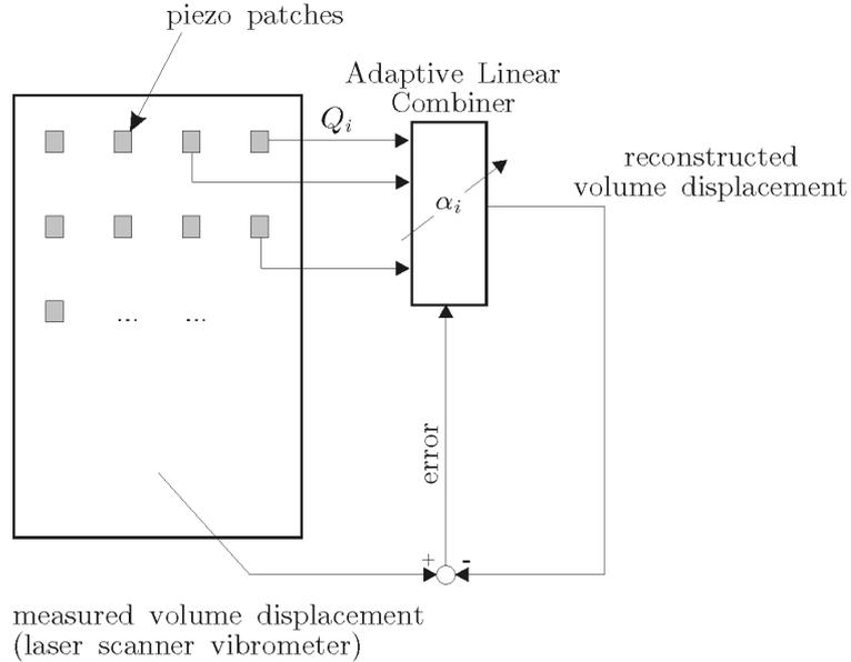
Figure 1: Principle of the volume displacement sensor
