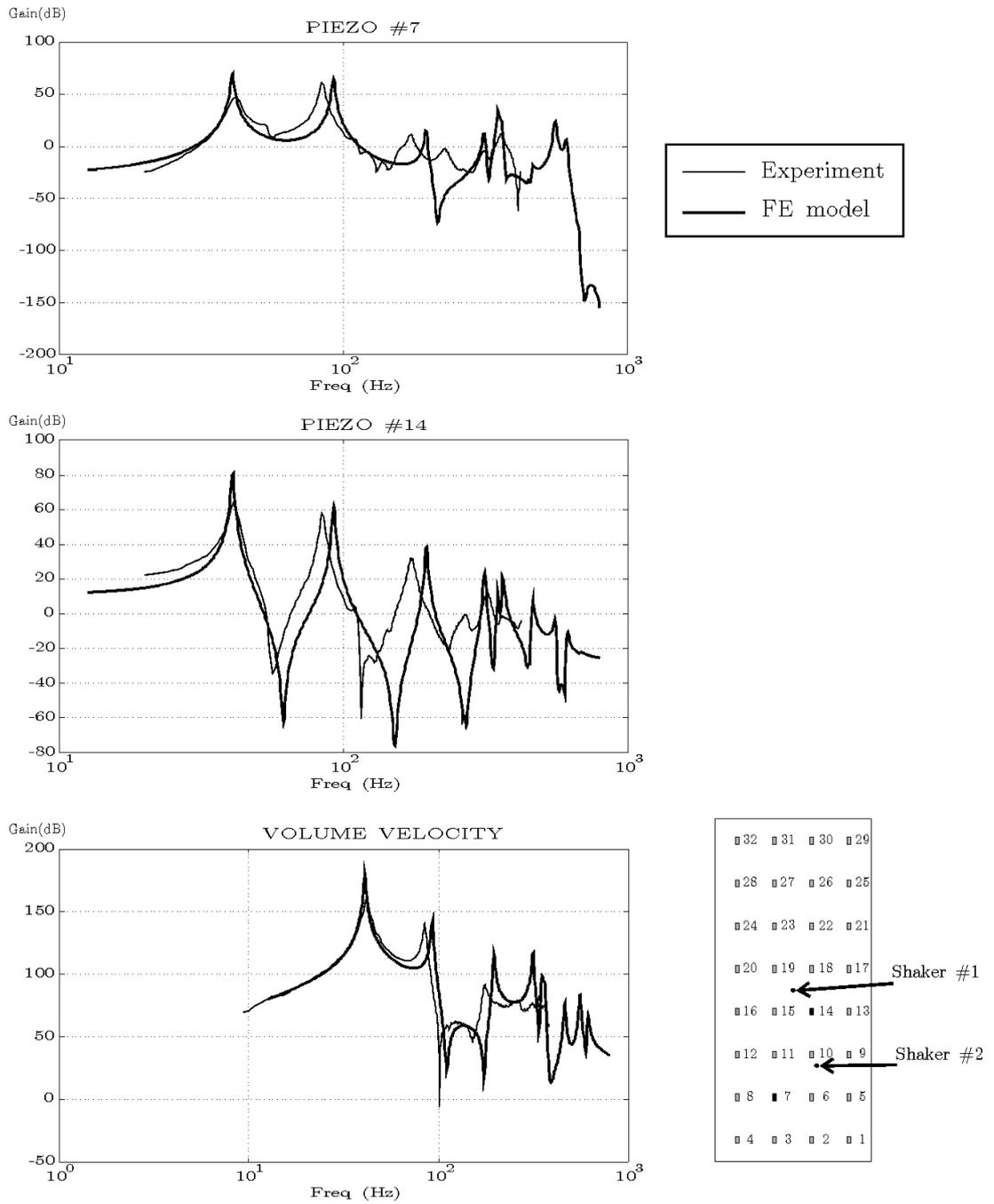
Figure 4: Frequency response functions /Shaker #1
