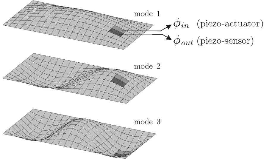
Figure 1: Piezoelectric elements location and first vibration modes
