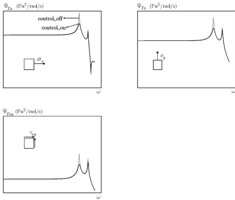
Figure 3: *PSD* of the stress components in the center of the plate with and without control
