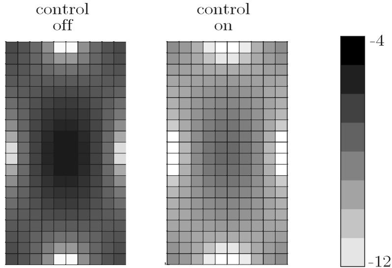
Figure 2: Damage map (Von Mises) with and without control (Log Scale)
