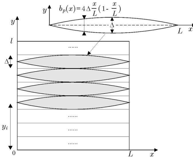
Figure 1: Discretisation of the active plate into narrow quadratic devices
