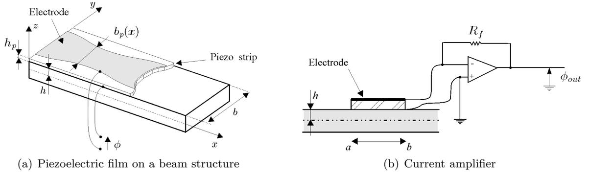
Figure 2: Piezoelectric beam device
