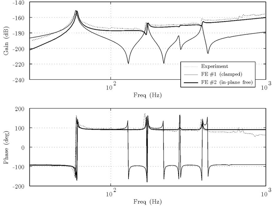
Figure 6: Open loop frequency response functions of the *ASAC* plate
