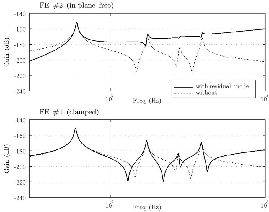
Figure 7: Effect of the residual mode (in addition to the 20 modelled modes) on the predicted open-loop frequency response functions
