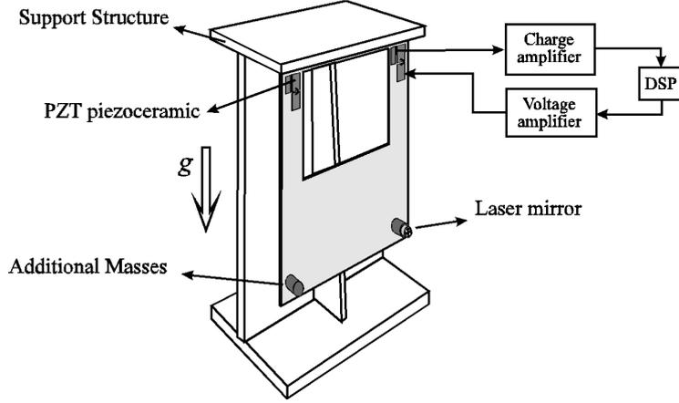
Figure 1: Laboratory demonstration model of the *CFIE* experiment.
