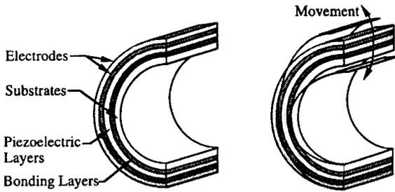
Figure 1: C-block actuator
