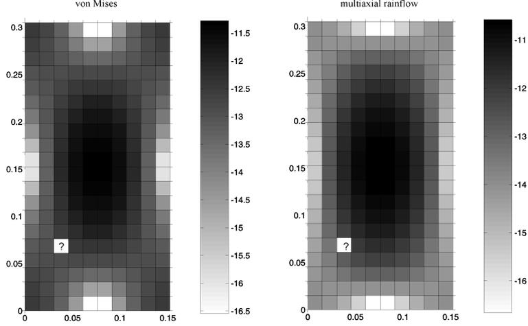
Figure 2: Map of the fatigue damage per time unit of the aluminium rectangular plate
